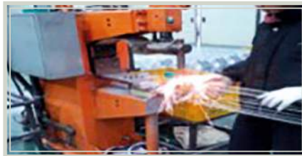
Cap Welder m/c
