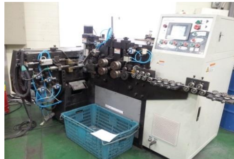
Automatic ring cutting and welding machine
