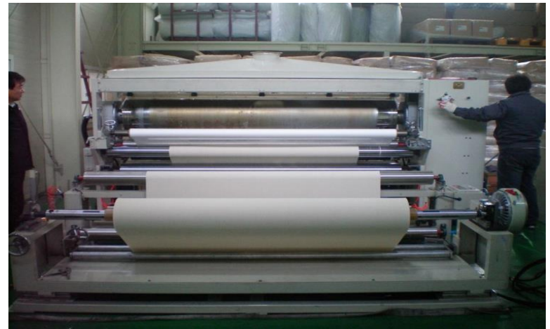
Laminating Unit 2 (2400mm Line)
