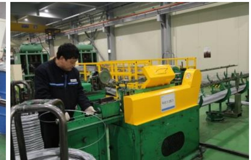
Straightening wire rods
